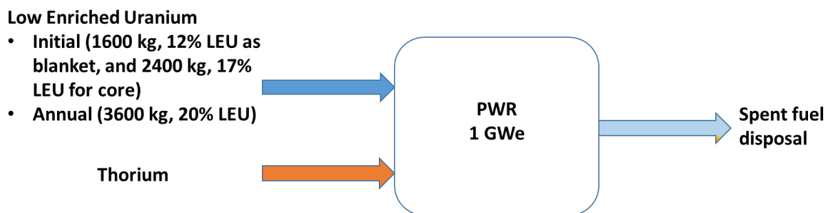
Figure 6: Thorium utilisation in PWR
