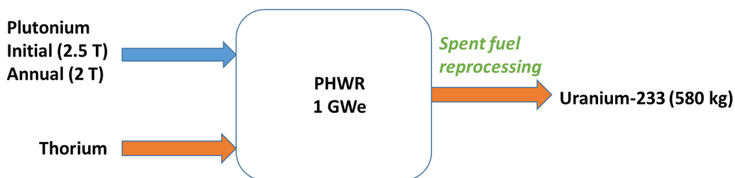
Figure 2: PHWR in thorium utilisation mode with Pu driver
