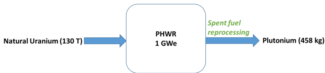
Figure 1: PHWR as the first stage of the three-stage programme
