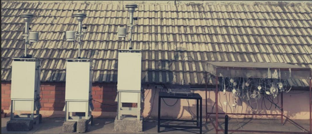
Sensors being calibrated against CSTEP BAM facility
